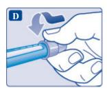
• **Pull off the outer needle cap and keep it for later.** You will need it after the injection, to correctly remove the needle from the pen.
