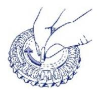
You can only turn the transparent dial after the tablet in the opening has been removed.
