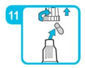
Unscrew mouth piece and remove the capsule from the chamber. Inspect the used capsule. It should appear punctured and empty.
