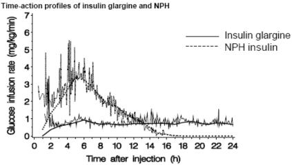
Mean GIR in subjects with type 1 diabetes mellitus after a single sc injection of 0.3 IU/kg insulin glargine or NPH (hourly mean data [n = 20] derived from, and superimposed on, smoothed original clamp data [where  $n \ge 5$ ] obtained at intervals of about five to ten minutes)
